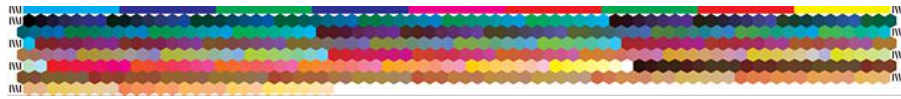
Figure 8-3 A roll-paper format that minimizes paper use by printing across the full width of the roll
